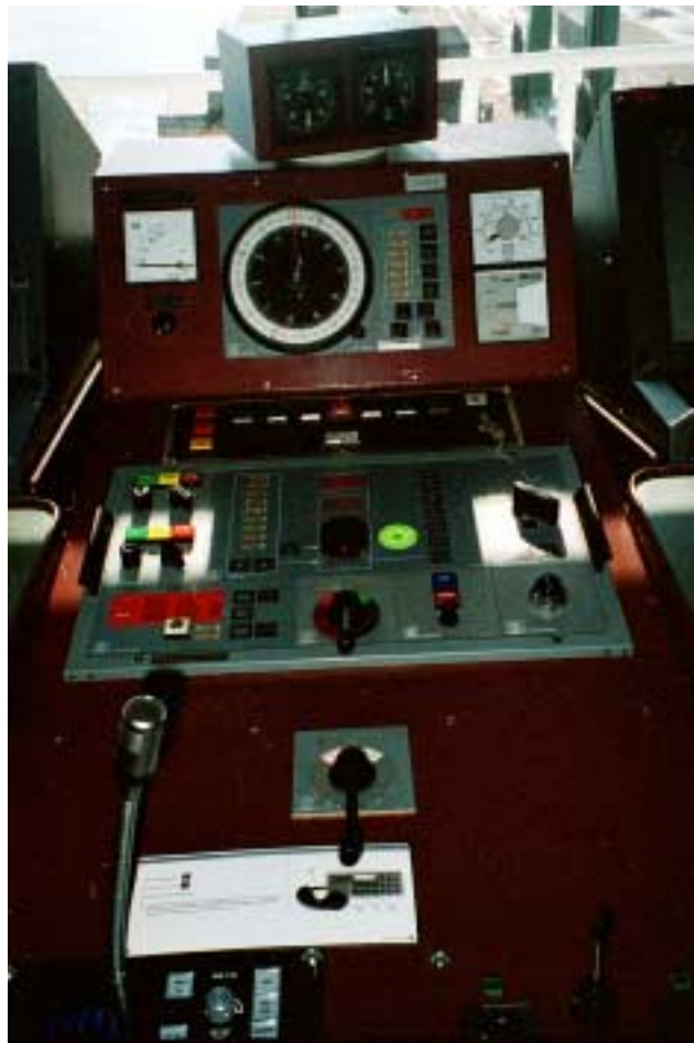
Figure 8. Middle cockpit console with autopilot and rate-of-turn and rudder-angle indicator (see also Figure 6).
