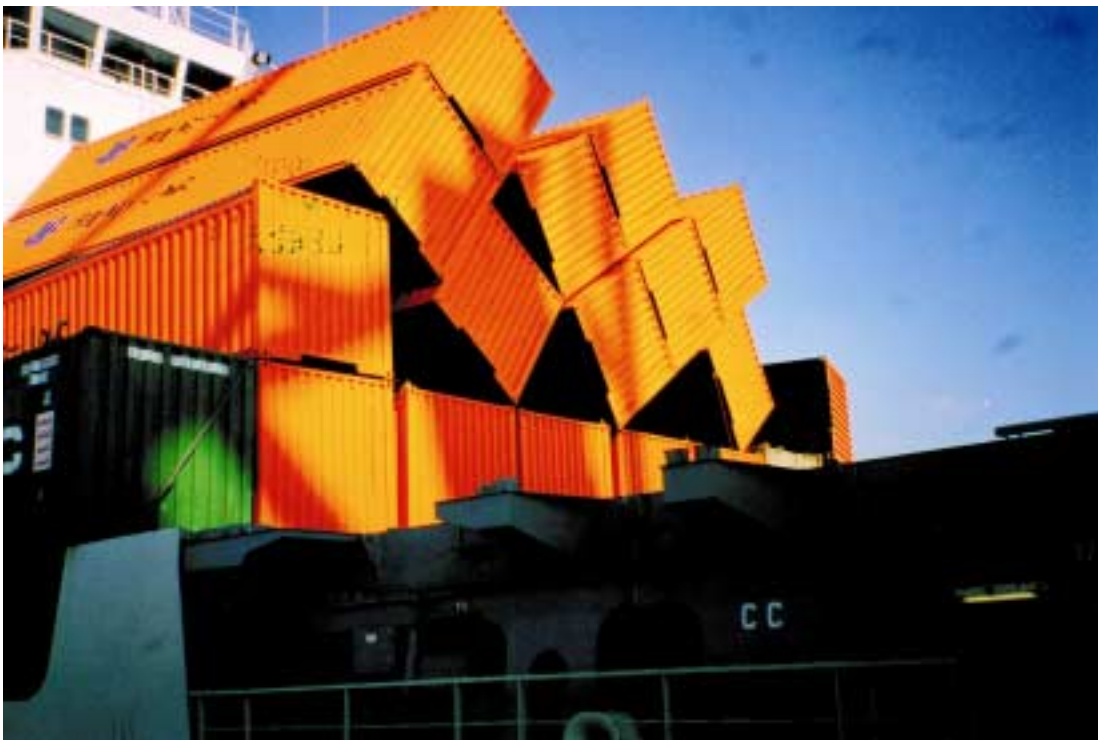
Figure 5. Stack of containers in front of bridge collapsed on impact. Four containers rolled overboard.
