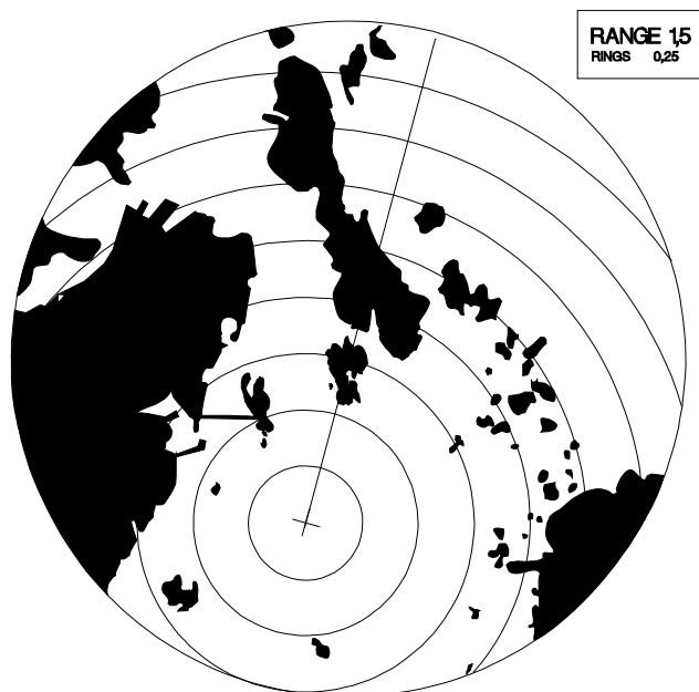
Figure 18. Range of radar 1,5', distance to Pirköyri 0,6'. Turn should have begun here.
