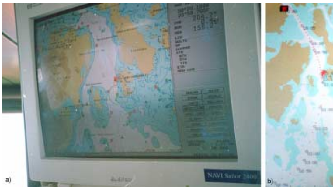
Figure 12. a) Monitor for electronic chart mounted in the ceiling (see also Figure 2).
